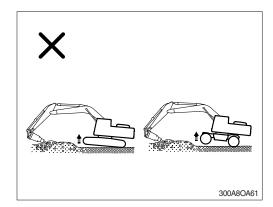
Excessive force as above may also result in vibrations being transmitted to the tracks causing damage.
